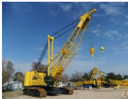
Gambar 4. 5 Alat crawler crane
