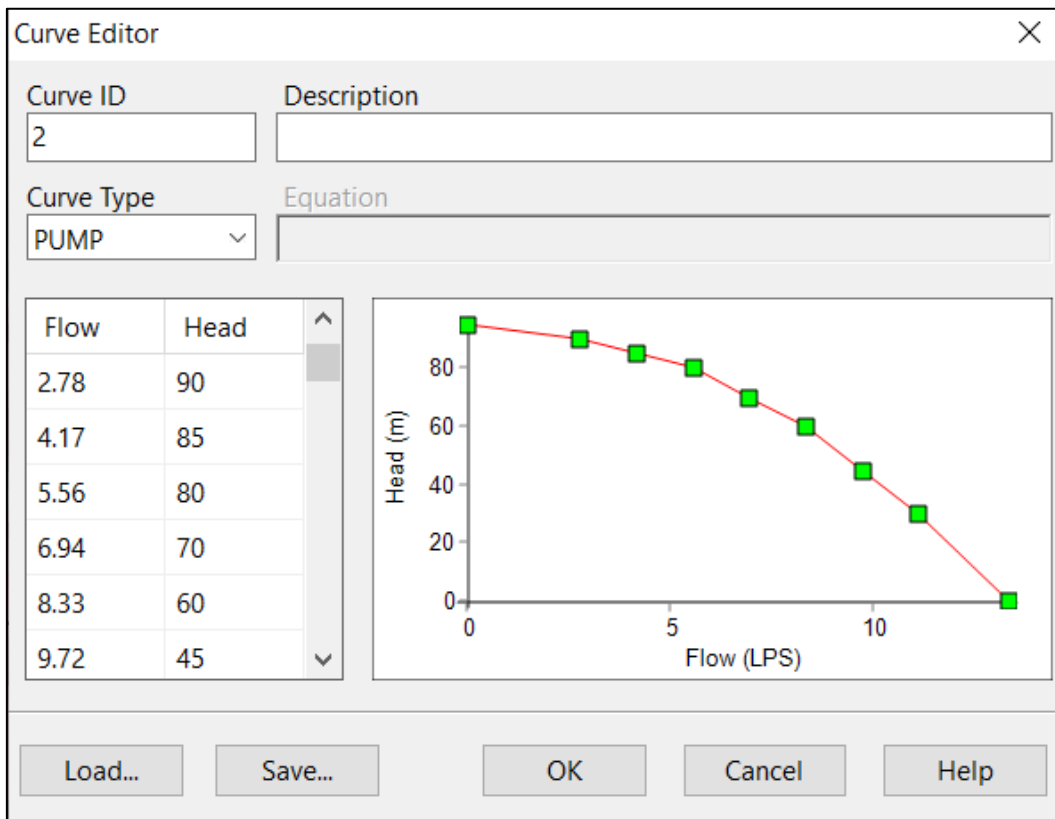
Gambar 4.2 Kurva Pompa Submersible Merk Vansan
