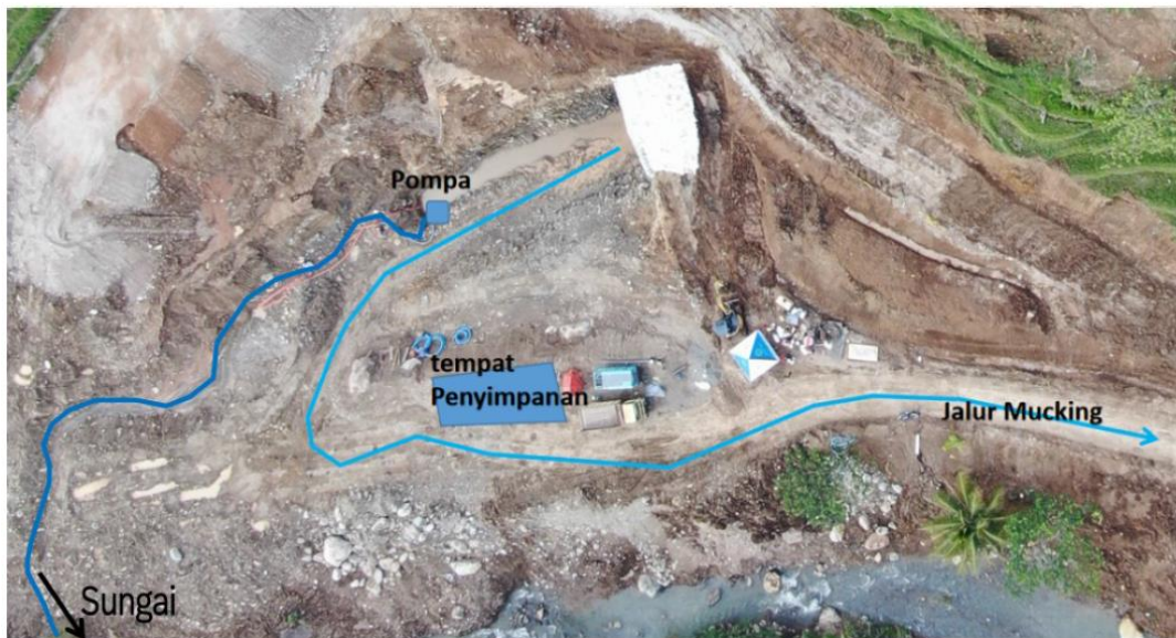
Gambar 3. 16 Ilustrasi Sistem Dewatering Outlet Tunnel
