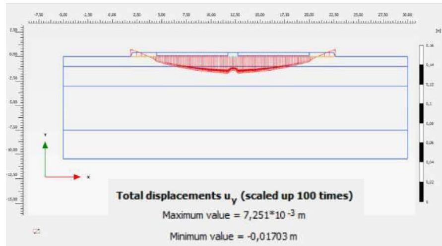
**Gambar 4.17** Output elevasi Potongan (A-A) tanpa perkuatan *water cement grouting*
