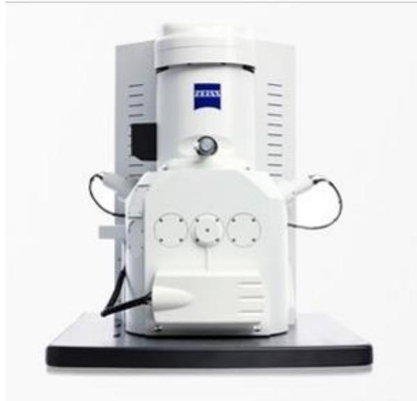
Gambar 3.2 Instrumen SEM-EDX
