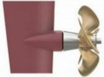
Gambar 2.3. Integrated Propeller & Rudder Sumber: (Ridwan, M. 2009)
