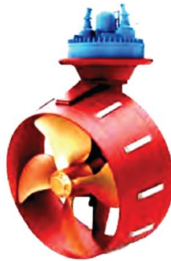
Gambar 2.4 Azimuth Thruster Sumber: (Budashko, V. 2017)
