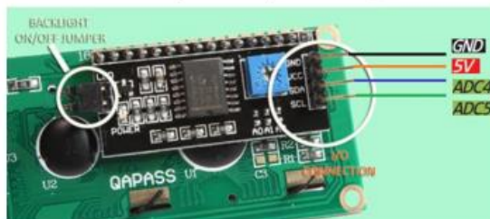
LCD display to Arduino wiring.
