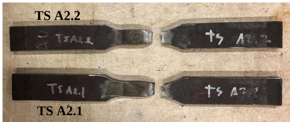
Gambar 4.7 Breaking Point Test Piece A2
