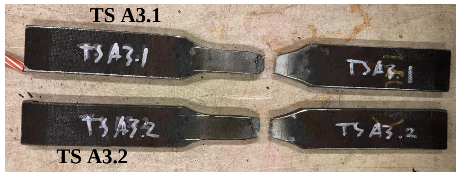
Gambar 4.8 Breaking Point Test Piece A3
