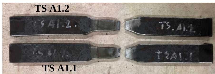
Gambar 4.6 Breaking Point Test Piece A1
