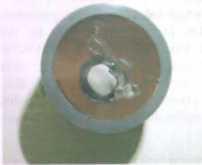
Gambar 3.7 Foto makro logam hasil peleburan 50 A, shielding gas Ar-He, 15 lpm
