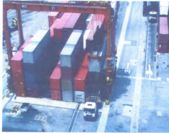
Gambar 2.3 Rubber Tyred Gantry Crane (RTGC) Sumber : Murty, Katta G.; Liu, Ji Yin; et al. (2005)
