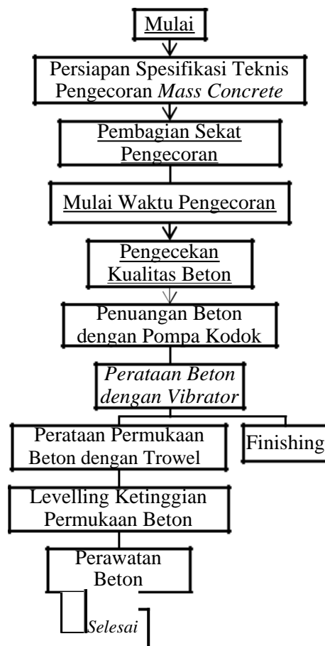
Gambar 2.44 Flowchart Pelaksanaan Pengecoran Mass Concrete
