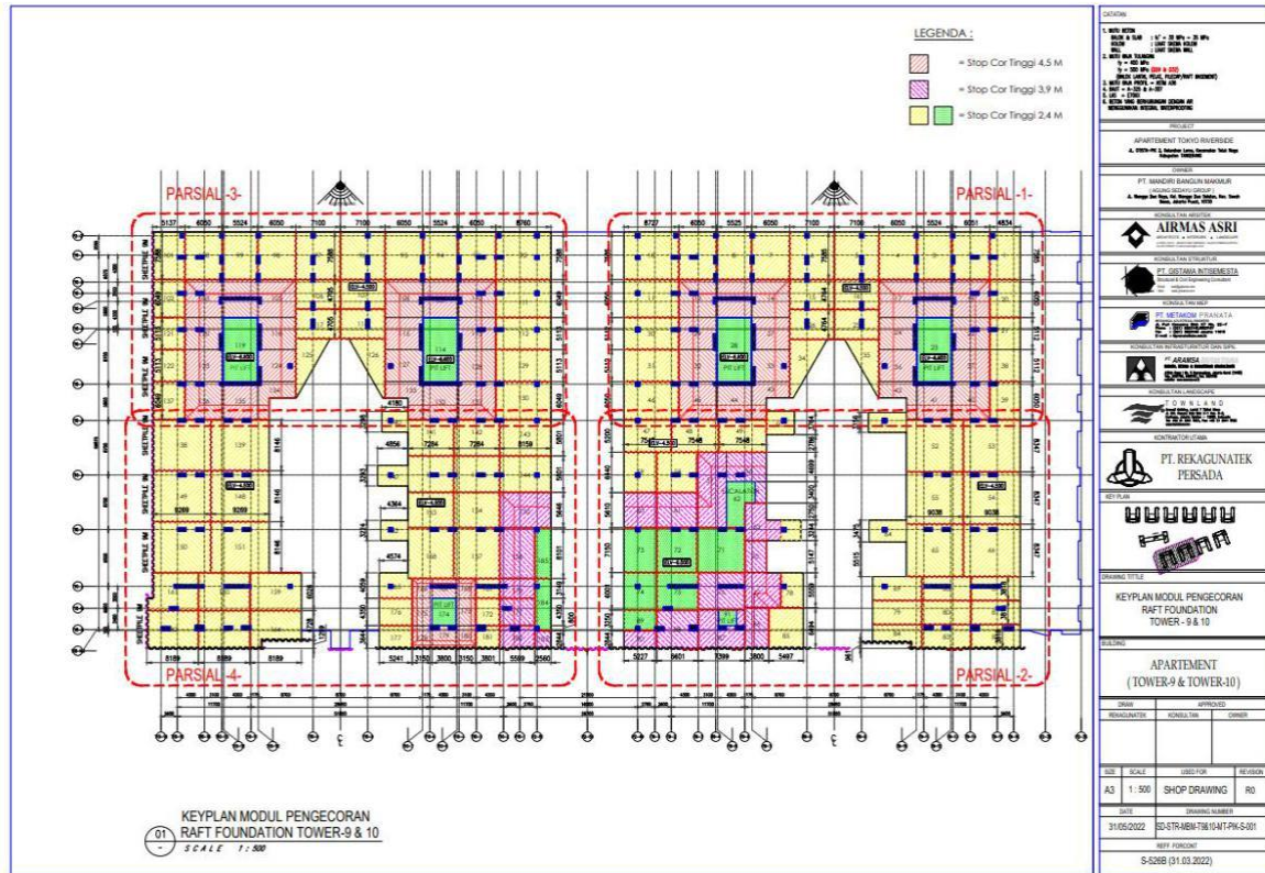
Gambar 4.1 Keyplan Modul Pengecoran Raft Foundation Tower 9 & 10
