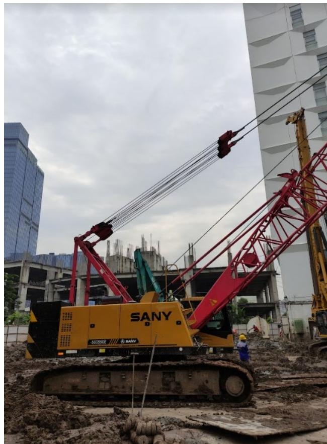
**Gambar 4.19 Crawler Crane SANY GROUP tipe SCC550E**
