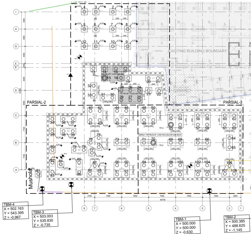
**Gambar 4.14 Denah Titik Pondasi Bore Pile**
