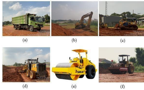
Gambar 2. 1 (a) Dump Truck, (b) Excavator, (c) Bulldozer, (d) Grader, (e) Vibrator Roller Compaction, (f) Sheep foot Tire Roller.
