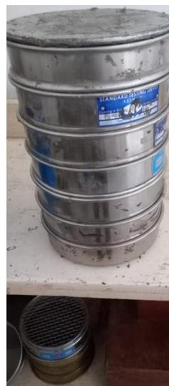
*Gambar 5.2 Saringan lolos agregat*
