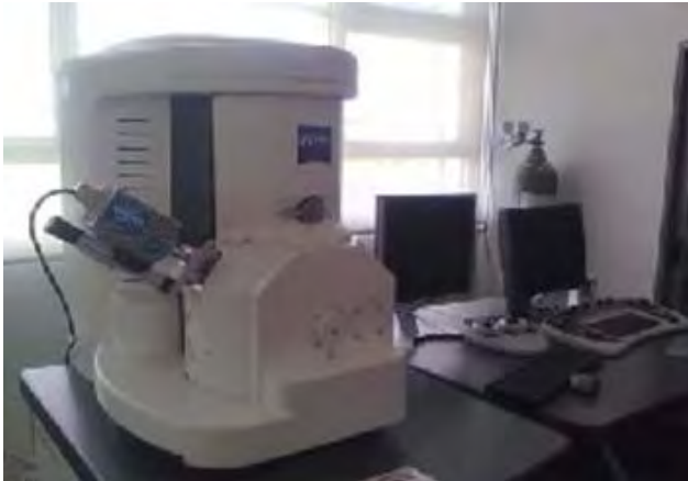
Gambar 3.8 Seperangkat peralatan SEM di laboratorium COE ( Center of Energy ) gedung robotika ITS Surabaya.
