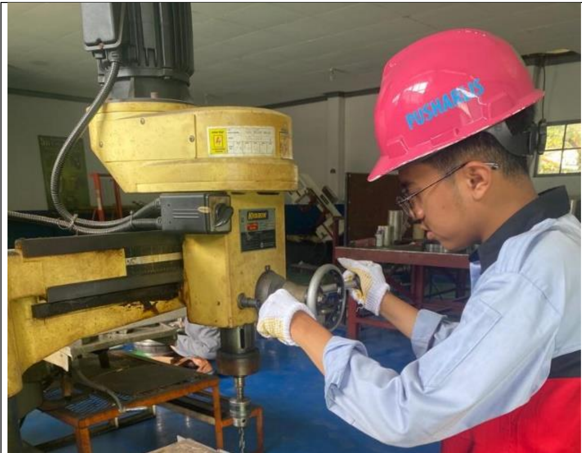
Drilling komponen Shuttle Trolley
