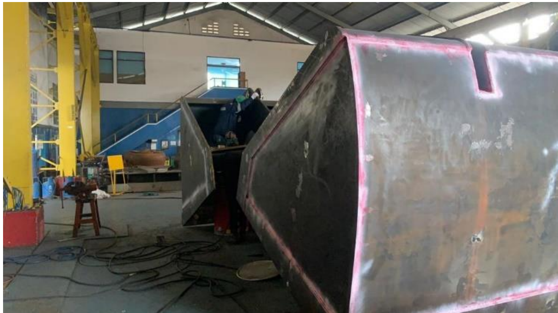
Gambar 4. 14 Grab Bucket Sebelum Proses Painting
