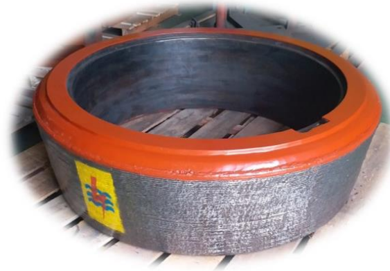
Gambar 2. 11 Grinding Tyre Pulverizer Coal Mill (Sumber : pln-pusharlis.co.id)
