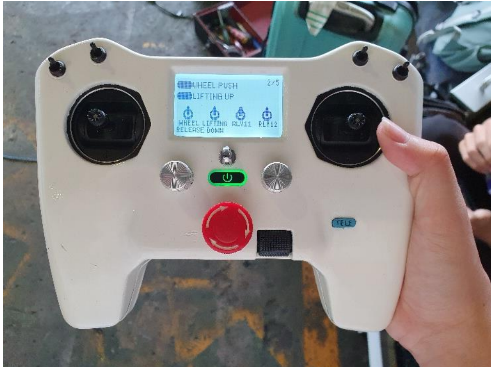
Prototype remote control berbahan PLA+
