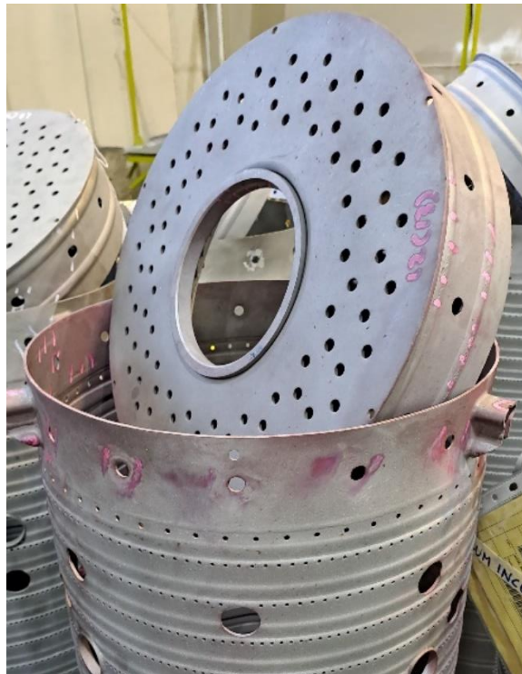
NDT komponen gas turbine di unit power services
