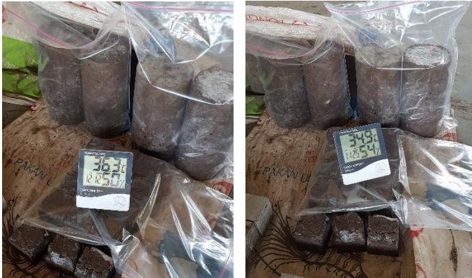
Gambar 3. 18 Suasana Perawatan Mortar Geopolimer
