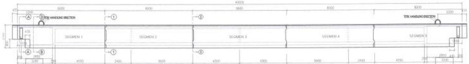
Gambar 4.31. Tampak Samping Girder A1-P1 Bentang 40 m
