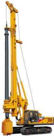
Gambar 2.2. Bore Pile Sumber : Google Image
