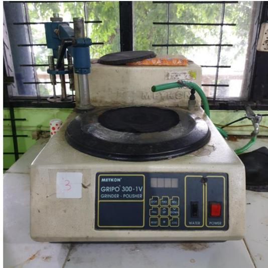
**Gambar 3. 5 Mesin Metkon GriPO 300-1V Grinder & Polisher**
