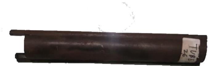
**Gambar 3. 2 Material Uji Pipa Baja SA 210 A1**
