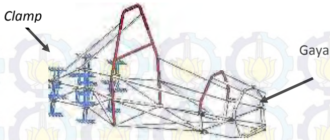
Gambar 2.15 Statik Shear (Singh, 2010)
