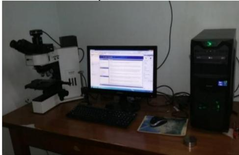
**Gambar 3.3** *Olympus Stereo Microscope*
