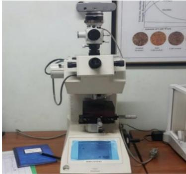
**Gambar 3.6** *Micro Hardness Vickers*
