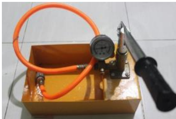
Gambar 3.8 Hydraulic Pressure Test
