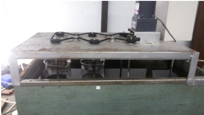
Gambar III.1 Waterbath reactor fungal treatment
