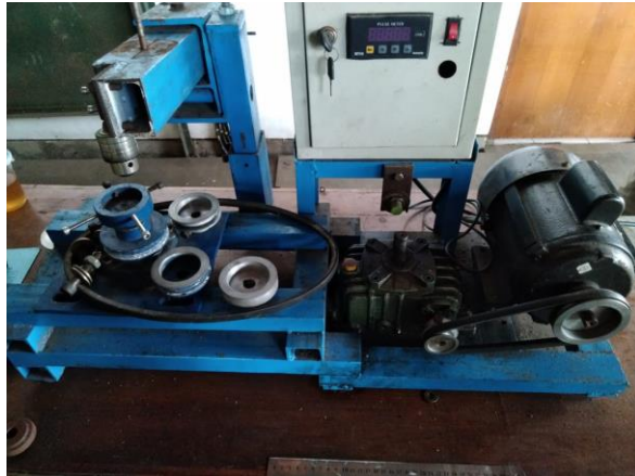
Gambar 3.6 Tribometer Pin on Disc
