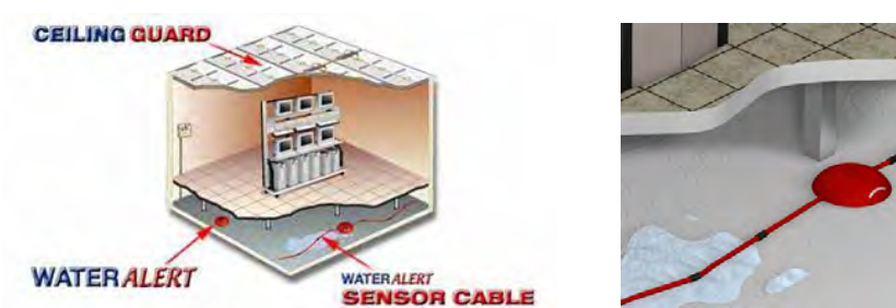
Gambar 6.8: water leaking detector
