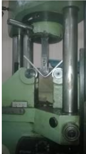
Gambar 3-12 Proses uji bending
