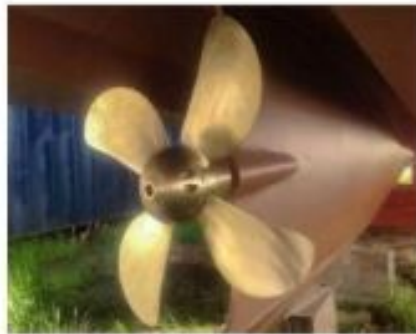
Gambar 4.3 Controllable Pitch Propeller (CPP)
