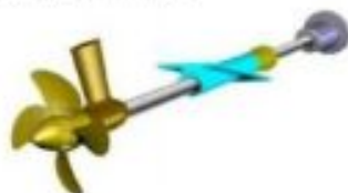
Gambar 4.2 Fixed Pitch Propeller (FPP)
