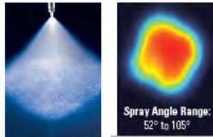
Gambar 25 hasil injeksi Full Cone (Square Spray) Nozzles type
