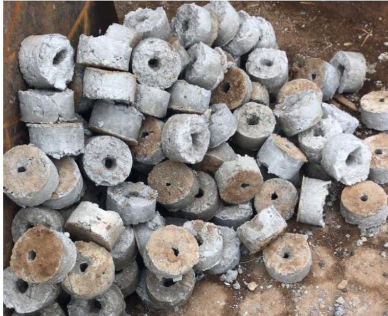
Gambar 3.11 *Decking* Beton
