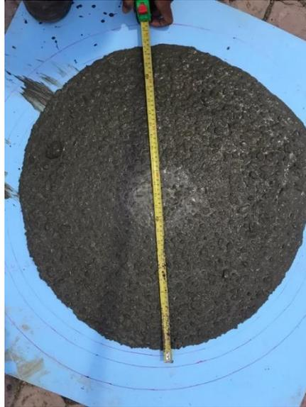
Gambar 3.16 Hasil *Slump Flow Test* Beton
