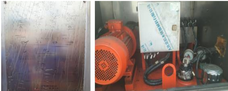
Gambar 4. 30 Power Pack Sistem Hidrolik Trim, List, Skew (TLS) di snag load
