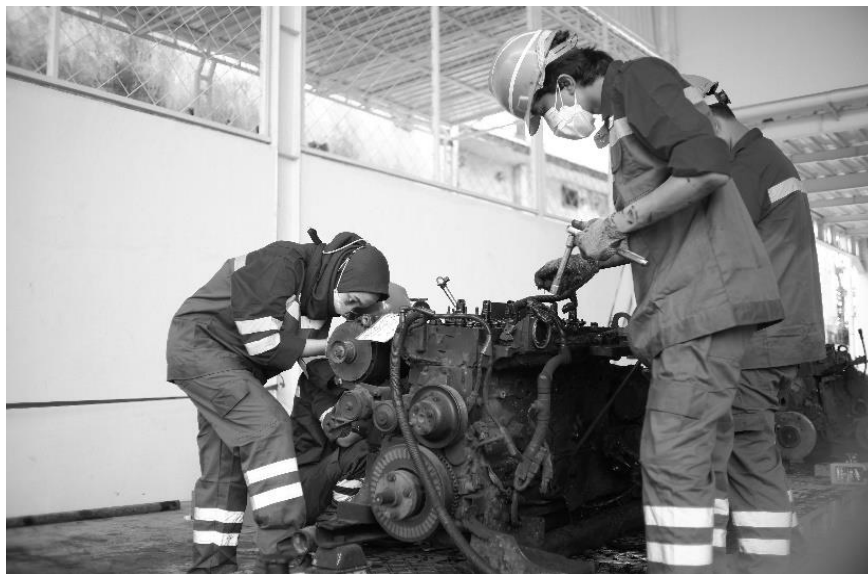
Gambar 4. 59 Overhaul Engine CTT di Workshop PT BIMA
