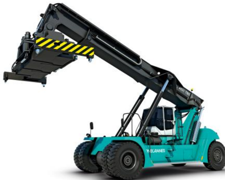
Gambar 4. 3 Reach Steaker Konecranes SMV 4127-4545 (Sumber : Konecranes maintenance manual, 2014)
