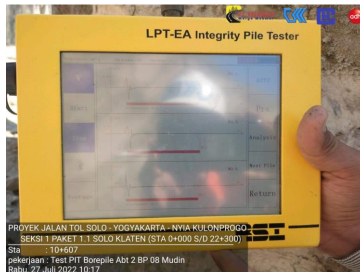
Gambar 3. 11 Pekerjaan Pile Integrity Test (PIT)
