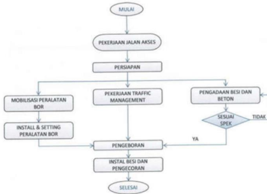
Gambar 3. 2 Flow Chart Pekerjaan Bore Pile
