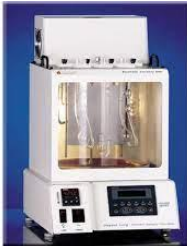
Gambar 3. 22 Alat uji viskositas ( viscometer bath )
